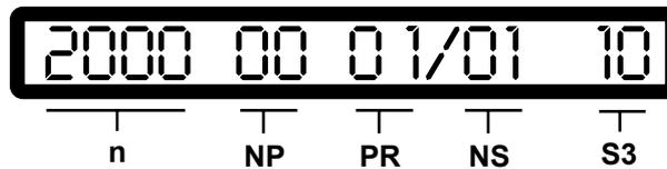
Programming of the **speed n** for the program (PR) is made via key A+ (value increased) or A- (value decreased)
