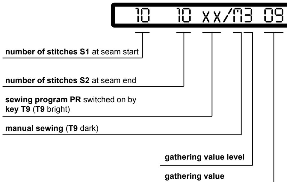
Following adjustments are possible only when the machine is stopped
