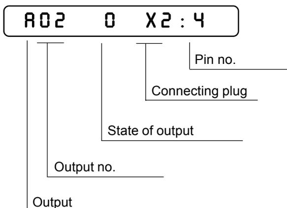
The function assigned to the output displayed can be seen from chapter 12 „Connections Diagram for Connectors“.
