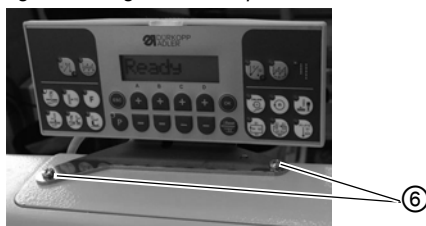
Fig. 41: Fitting the control panel - Part 2
