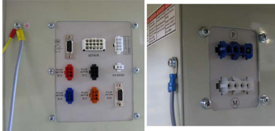
Fig. 25: Connecting the cables to the control unit
