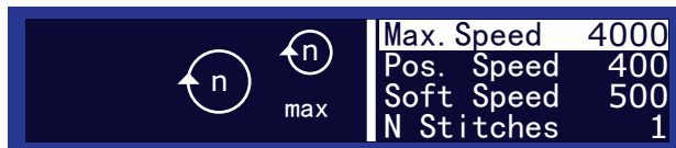
Figure 51: Parameters in the submenu Speed
