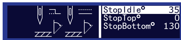
Figure 52: Parameters in the submenu Stop Positions
