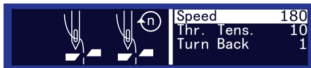
Figure 50: Parameters in the submenu Thread Trim
