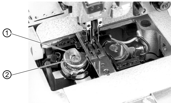
(1) - Upper part bobbin case (2) - Bobbin case flap
