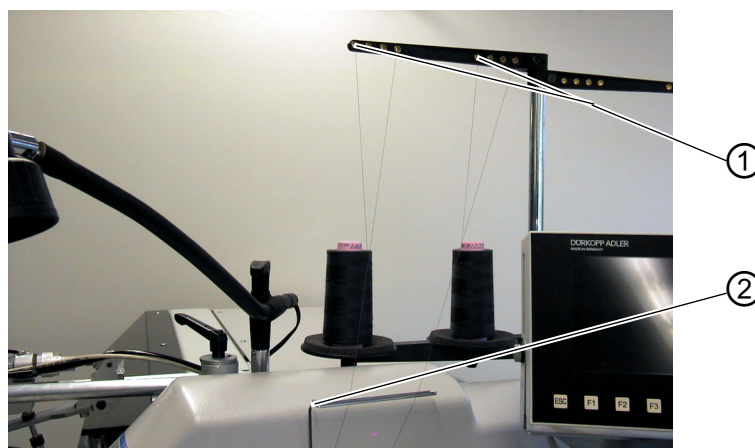
(1) - Drill hole (thread reel holder)
