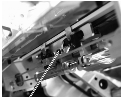
① (1) - Cutting unit (2) - Stop
