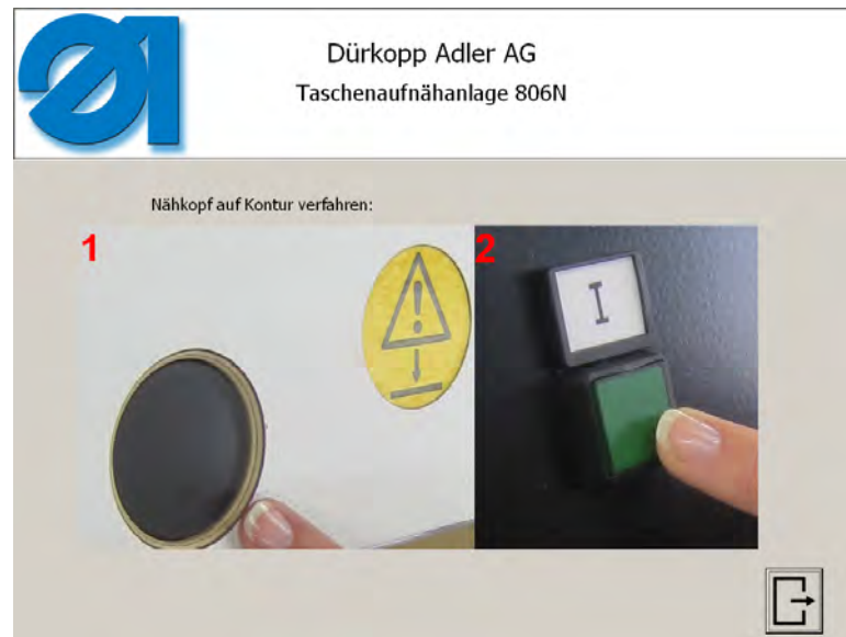
Figure 53: Message after thread breakage
