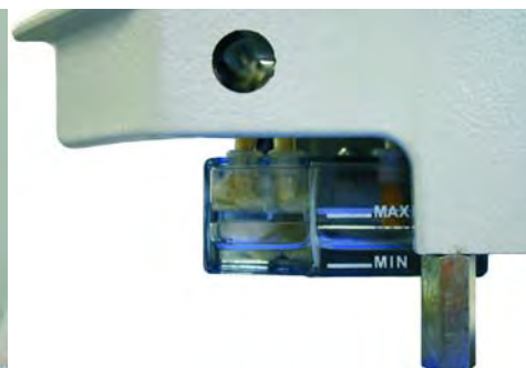
Oil reservoir 2 - under the sewing material support
