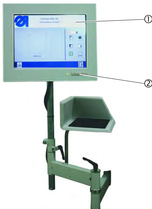
Figure 2: Overview of the operating terminal
