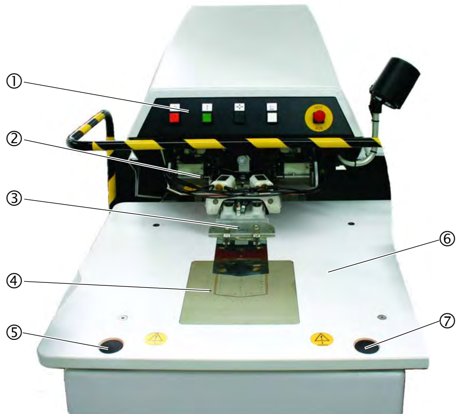
Figure 3: Overview of the edge folding station
