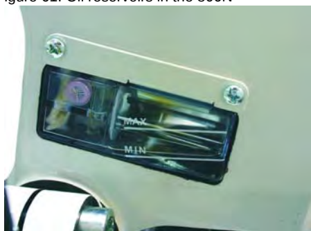
Figure 61: Oil reservoirs in the 806N
