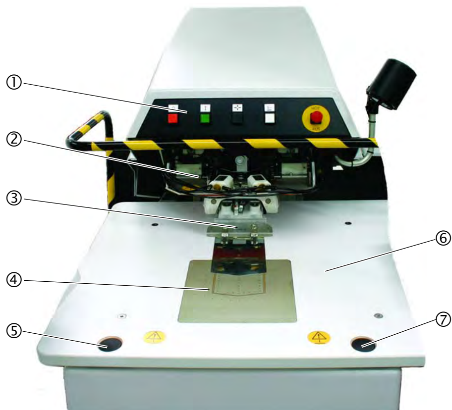
Figure 37: Overview of the edge folding station
